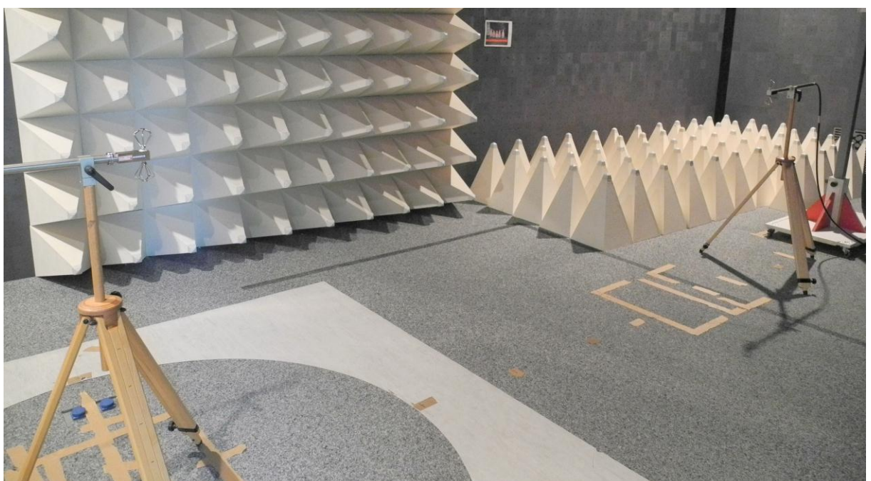
Figure 2: Calibration setup using a 2 nd antenna (on left side)
